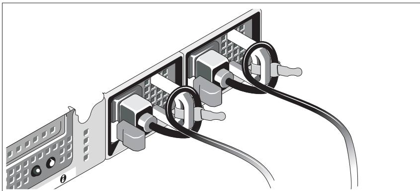
Bend the system power cable(s) into a loop as shown in the illustration and secure the cable(s) to the bracket using the provided strap. Plug the other end of the power cable(s) into a grounded electrical outlet or a separate power source such as an uninterrupted power supply (UPS) or a power distribution unit (PDU).
